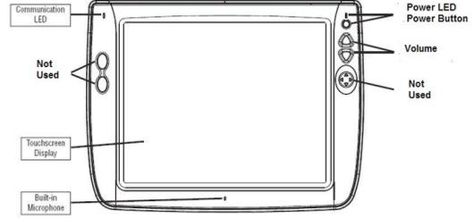
\*If the screen stays blank when touched, check the power LED in the upper right corner. The power button is located below the LED.
